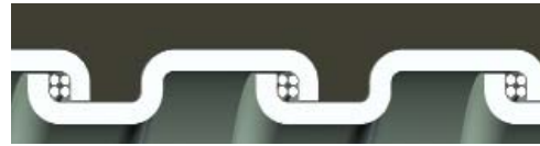
Square-Locked Design with cord packing 3/8" through 1-1/4"
