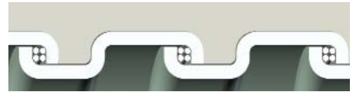
Square-Locked Design with cord packing 3/8" through 1-1/4"
