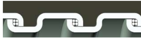
Square-Locked Design with cord packing 3/8" through 1-1/4"
