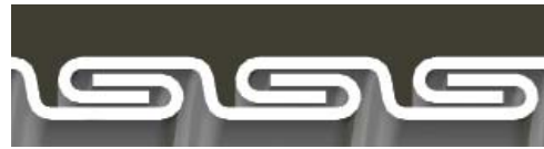
Interlocked Design 1-1/2" through 4"
