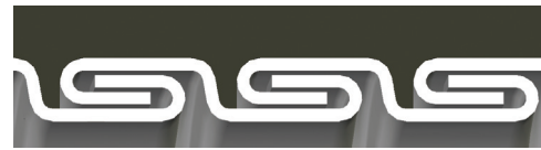
Interlocked Design 1-1/2" through 4" with no bonding wire
