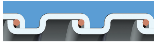
Square-Locked Design with integral bonding wire 1/2" through 1-1/4"
