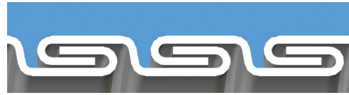
Interlocked Design 1-1/2" through 3" with no bonding wire
